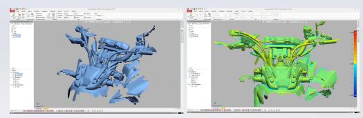
Application of the **3D scanning technology** using the **eviXscan 3D scanner** significantly shortens the whole production process and improves its quality, furthermore, it increases the repeatability and enables easy editing of the prepared models.
